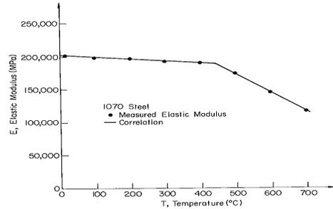
Figure 7 Elastic Modulus as function of temperature.
