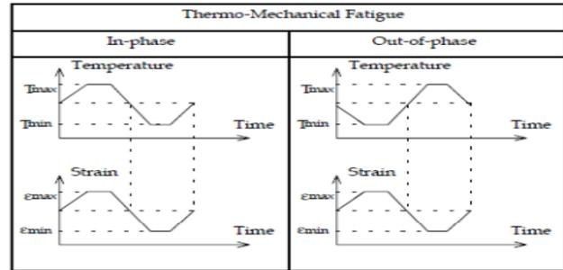
Figure 3 In-phase and Out-of-phase TMF loading patterns
