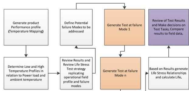
Figure 8 Test procedure
