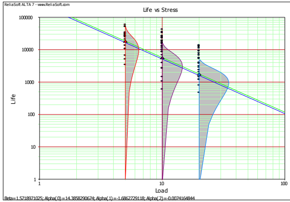
Figure 5 – Life-Stress Relationship Plot for Component A (Varying Load, Fixed Frequency = 250)
